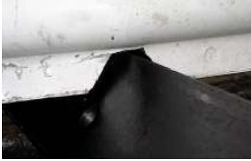
4. Slide cross member with center circular receiver notch cut out (Rear cross member) through notch (Open angle will face towards front of truck) and move towards back of truck. Other cross member can now be slide in (Open angle facing front of truck, same orientation as rear cross member).
