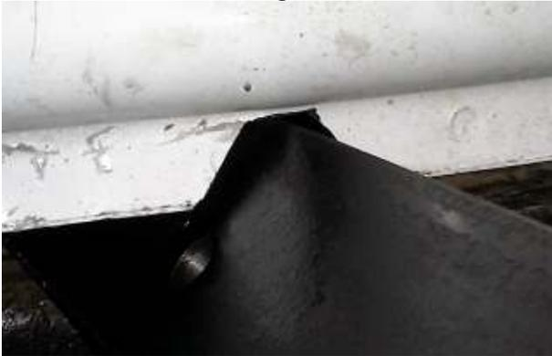
5. Slide front cross member through notch across truck frame with open angle facing towards back of truck. Move cross member towards front of truck. Now slide rear cross member in open angle facing back of truck (same orientation as front cross member)
