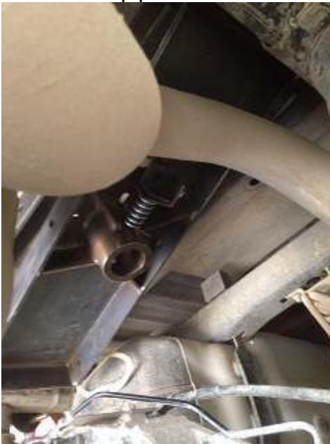
10. Install cross members to center plate with ½” bolts and lock washers and hex nuts. (Do not tighten).
