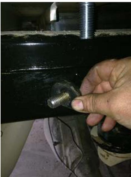
8. Pull bolt back through hole and slide spacer washer over bolt and insert it into the frame. Thread spring nut retainer clip on bolt and hand tighten to the frame to hold the bolt in place.
