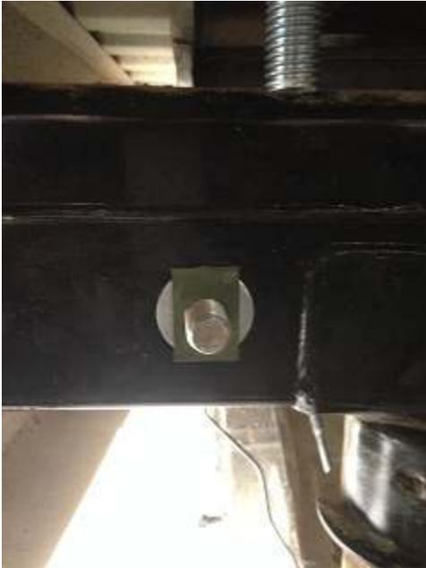
9. From underneath truck slide center plate in place from driver's side, up and over exhaust tail pipe.
