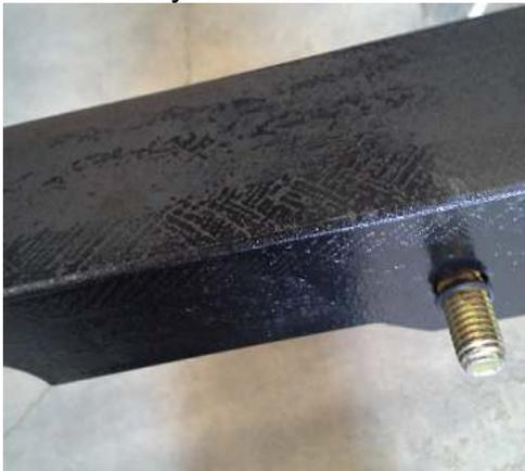
8. Install cross members to center plate with  $\frac{1}{2}$ " bolts and lock nuts. (Do not tighten.
